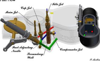
GREEN: Adjustable fuel supply for Cap Jet BLUE: Predetermined fuel supply by Compensator Jet for Cap Jet and Idle Jet RED: Direct fuel supply for Main Jet (Used for High Speeds)
