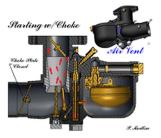
When the engine is started with the choke closed a greater vacuum is formed, pulling in a larger amount of fuel.
