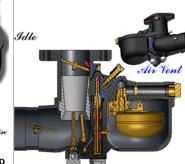
The "Compensating Jet" is inside the fuel bowl and empties into the "Secondary Well" which is open to the air. The "Cap Jet" connects with the "Secondary Well". The "Cap Jet" can only draw as much fuel as the "Compensating Jet" will allow, regardless of the amount of suction.
